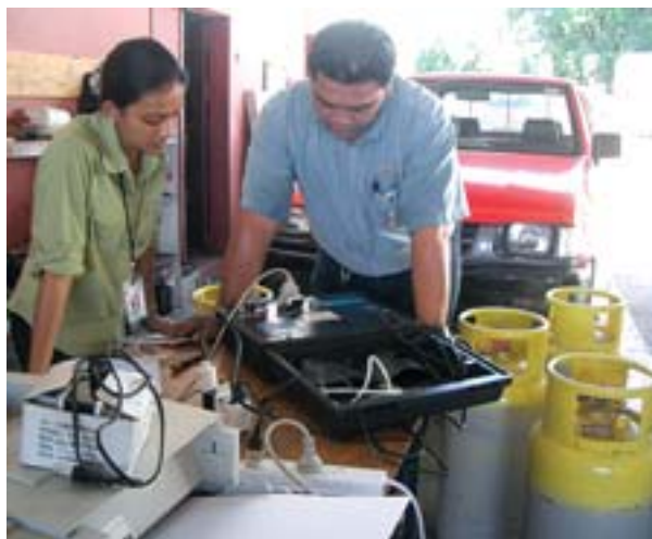
Philippines Customs Officers using refrigerant identifier to check imported ODS
